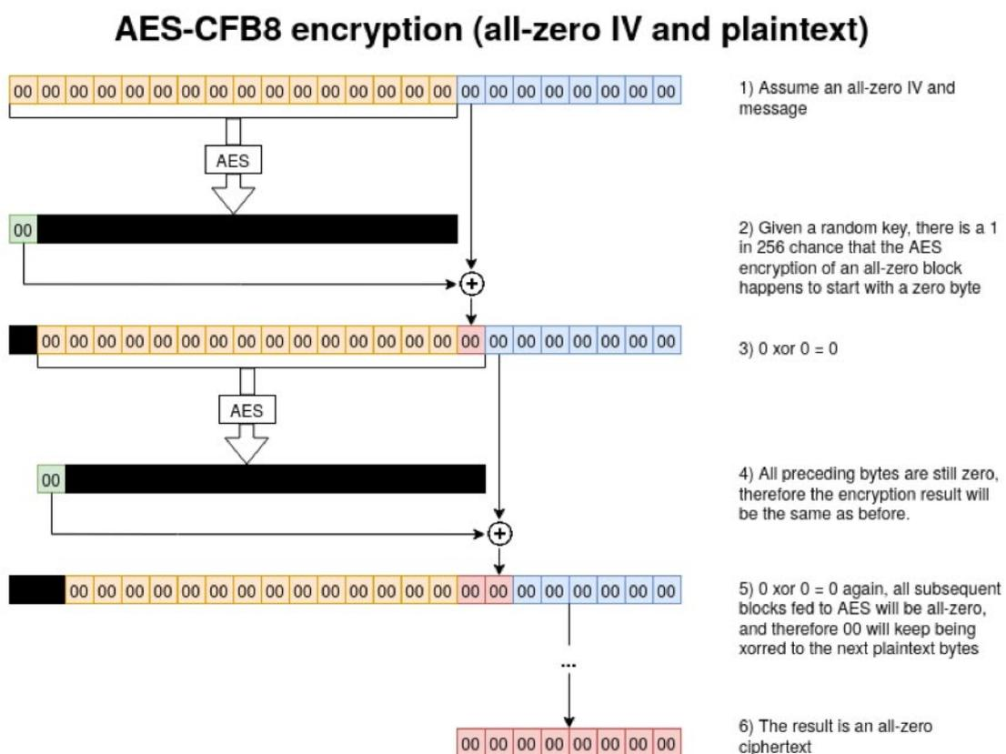
Figure 3: When encrypting a message consisting only of zeroes, with an all-zero IV, there is a 1 in 256 chance that the output will only contain zeroes as well.
